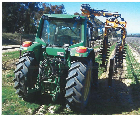
A tractor mounted mechanical pruner. The cutter removes the trellised shoots above the horizontal cordon.
